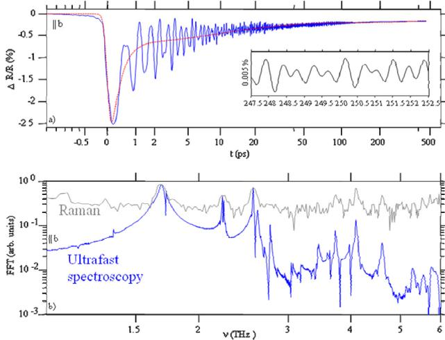
**Figure 1.** Panel a) shows the transient change in reflectivity after excitation with a 50 fs laser pulse of 800 nm central wavelength. The inset shows the magnified signal 250 ps after excitation which still shows strong oscillations. In b) the oscillatory signal has been Fourier transformed (blue). The data is compared to the recent Raman data (grey).[6]
