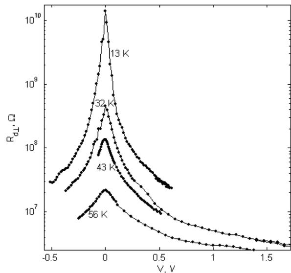
**Figure 3.** Voltage dependences of the transverse differential resistance of a  $\text{TiS}_3$  whisker at various temperatures.
