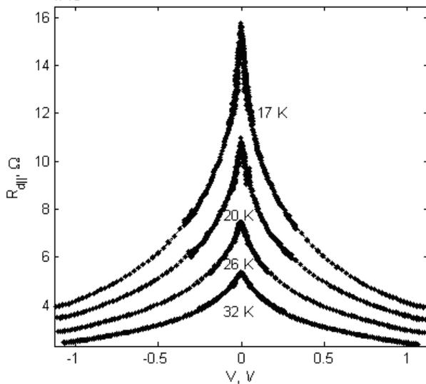
**Figure 2.** Voltage dependences of the longitudinal differential resistance of the  $\text{TiS}_3$  whisker at various temperatures.
