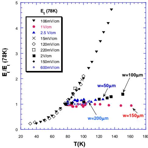
Figure 3. Threshold field as a function of temperature normalized to the threshold at 78 K for bulk samples and needles.
