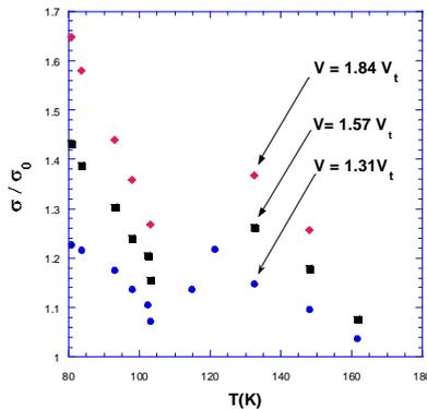
Figure 4. Normalized conductivity vs temperature for different values of the dc voltage.
