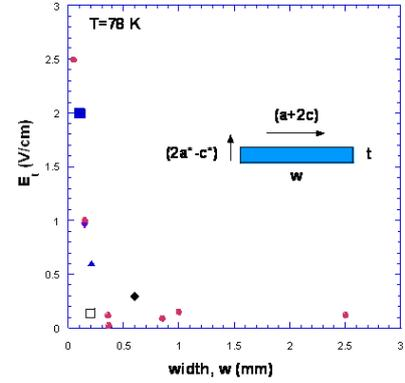
Figure 1. Threshold field at  $T = 78\text{ K}$  as a function of the width of the samples. ( $\blacklozenge$ ) from ref. [5].
