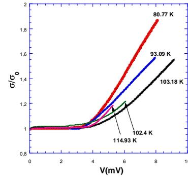
Figure 2 (a). Nonlinear conductivity normalized to the Ohmic conductivity at different temperatures vs dc voltage.
